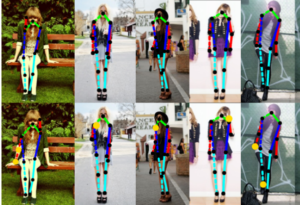
Figure 4: Human pose estimation with Decision Forests using the fertilized forests library (c.t. [14]). The samples are part of the FashionPose dataset [7].
